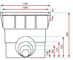
**Stormwater Pit** Code: 97965 Weight: 43kg
