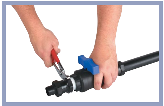
3. Do not over tighten. The recommended way to assemble a Ball Valve is finger tight. Tighten until firm with spanner or pipe grip. One to two turns should be all that is required.
